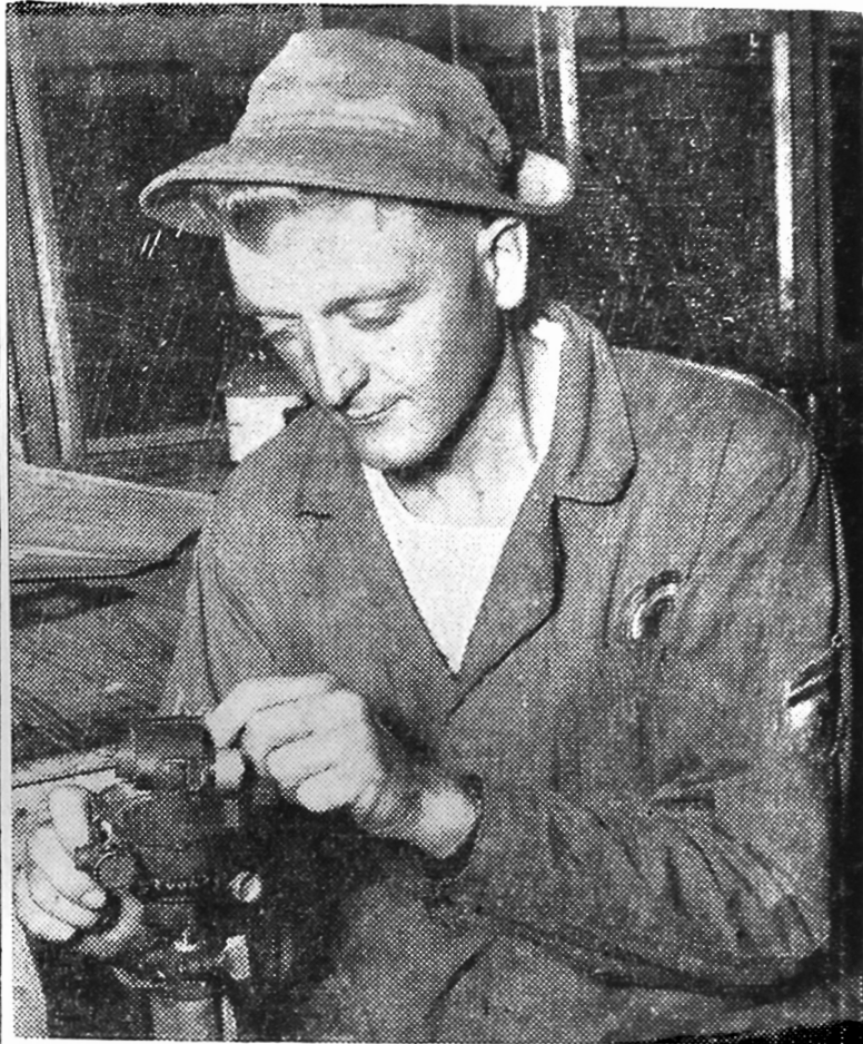
Heavy machine guns are laid on distant targets with the aid of the aiming circle. T-5 Kenneth E. Thompson, 742nd Ord. Co., is repairing one in MRS 12 where such repairs as can be done in the Division are carried out. (U. S. Signal Corps Photo.)
