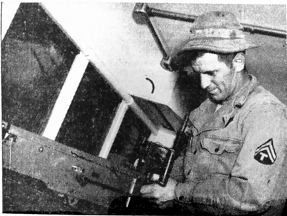
To save time and keep weapons in working condition at all times, the 742nd Ordnance Company operates a small arms repair truck on the ranges. T-5 James Creamer removes the backplate of a .50 caliber machine gun which he is repairing in the truck. (U. S. Signal Corps Photo.)
