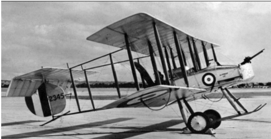
WWI-148 Vickers F.B.5 Gunbus, from ca. 1915. This was an early British fighter plane. Note the front mounted machine gun and the backward facing engine and propeller.
